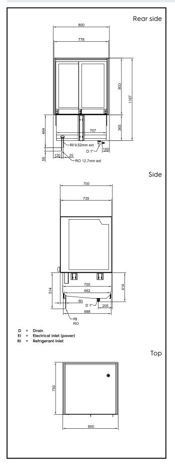
Drop-In Drop-in remote refrigerated well with refrigerated display, squared, medium service - 4 hours - 2GN The company reserves the right to make modifications to the products without prior notice. All information correct at time of printing.
