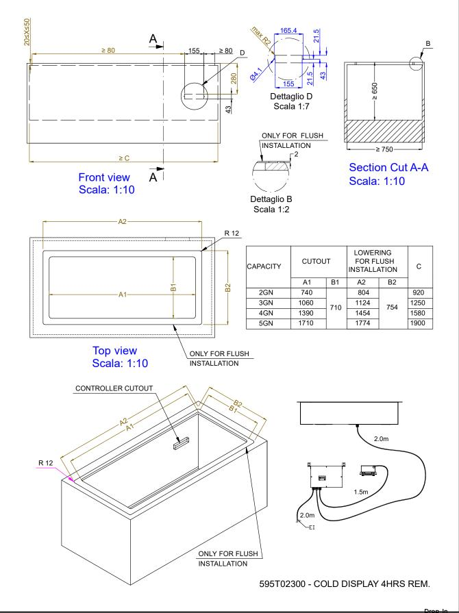
Drop-in Drop-in remote refrigerated well with refrigerated display, squared, medium service - 4 hours - 2GM The company reserves the right to make modifications to the products without prior notice. All information correct at time of printing.
